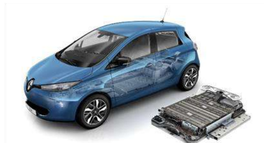
Zoé 400 V, 41 kWh, 12 modules, 192 cellules, 290 kg
